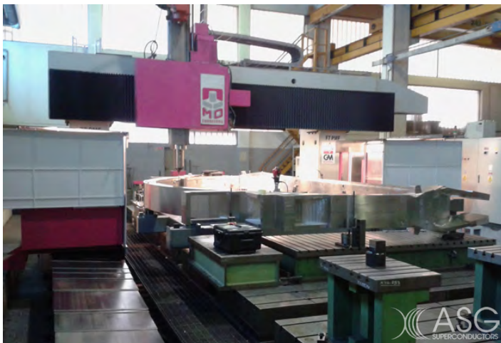
Figure 24 TFC interface machining (courtesy of Officine CLP)
