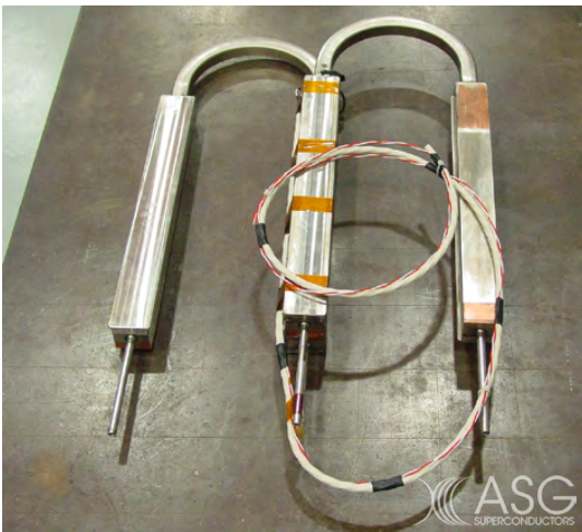
Figure 10 Full size joint sample tested by ENEA
