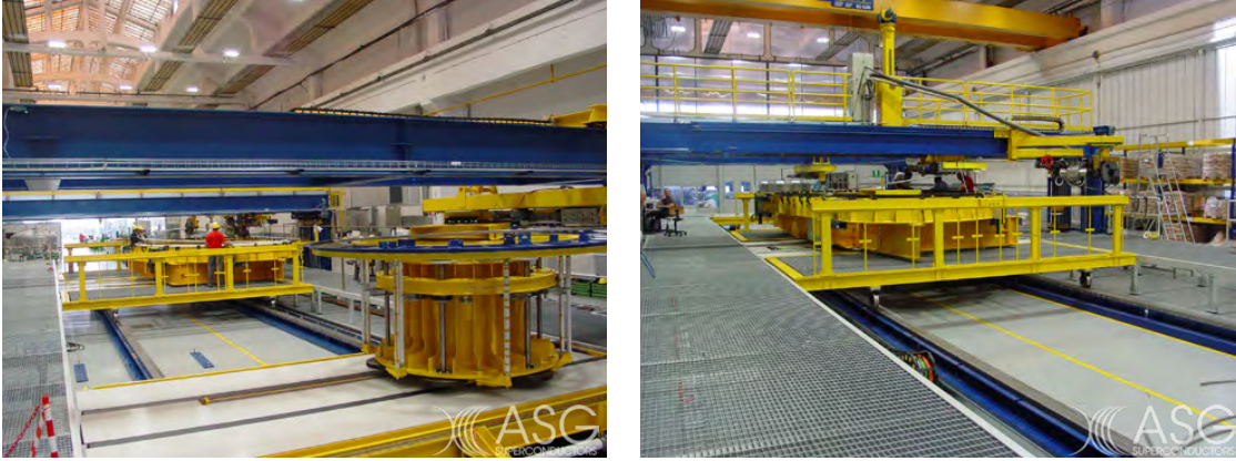
Figure 11, 12 Winding Line-Unwinding spool / Winding Line-Winding Table
