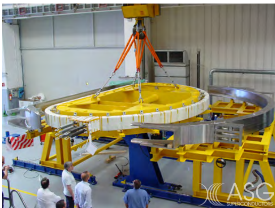
Figure 21, 22 WP and coil casing onto the assembly tooling / Assembly tilted in vertical position for welding execution
