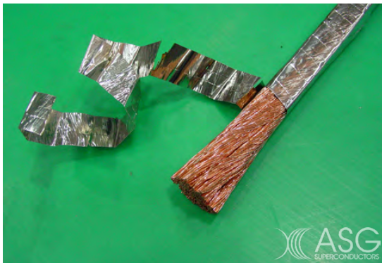
Figure 1, 2, 3 Details of the JT-60SA conductor
