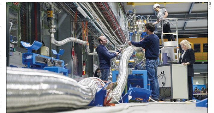
Link to the future Tests at CERN of a full-scale 120 kA MgB 2 -based superconducting link “Demo 3”, colloquially known as the “python”, for the High-Luminosity LHC.
