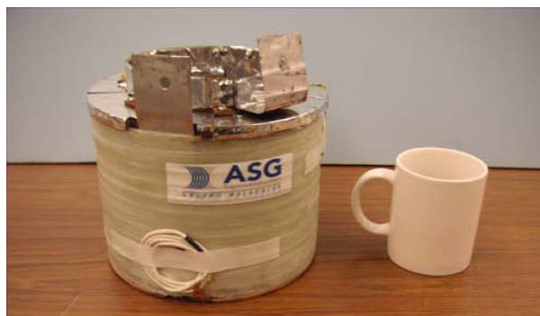
The 16K, 1 Tesla solenoid magnet realized with MgB_2 React & Wind conductor
