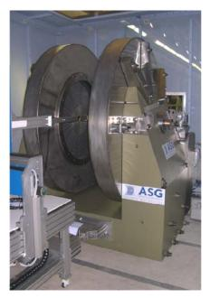
The ASG's MRI 0.5T cryogenic free magnet
