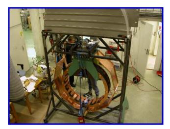
Superconducting coil under construction
