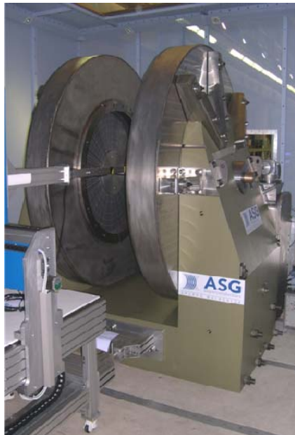
The ASG's MRI 0.5T cryogenic free magnet
