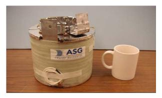
The 16K, 1 Tesla solenoid magnet realized with MgB $_2$  React & Wind conductor
