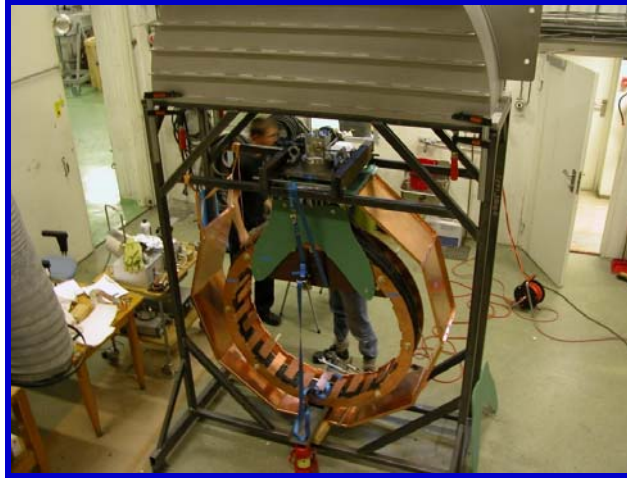
Superconducting coil under construction
